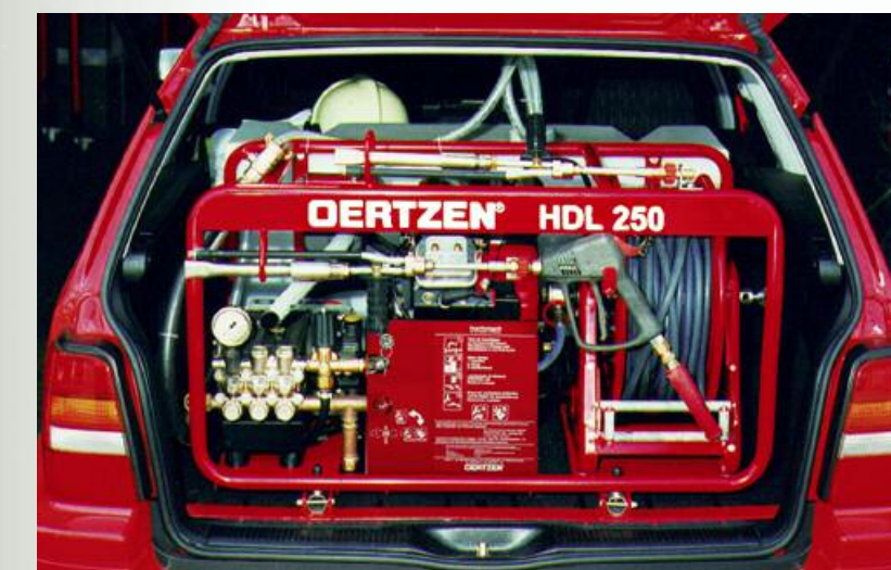
HDL 250 as compact installation unit installed in a small car with 125 liter tank in front of it.
